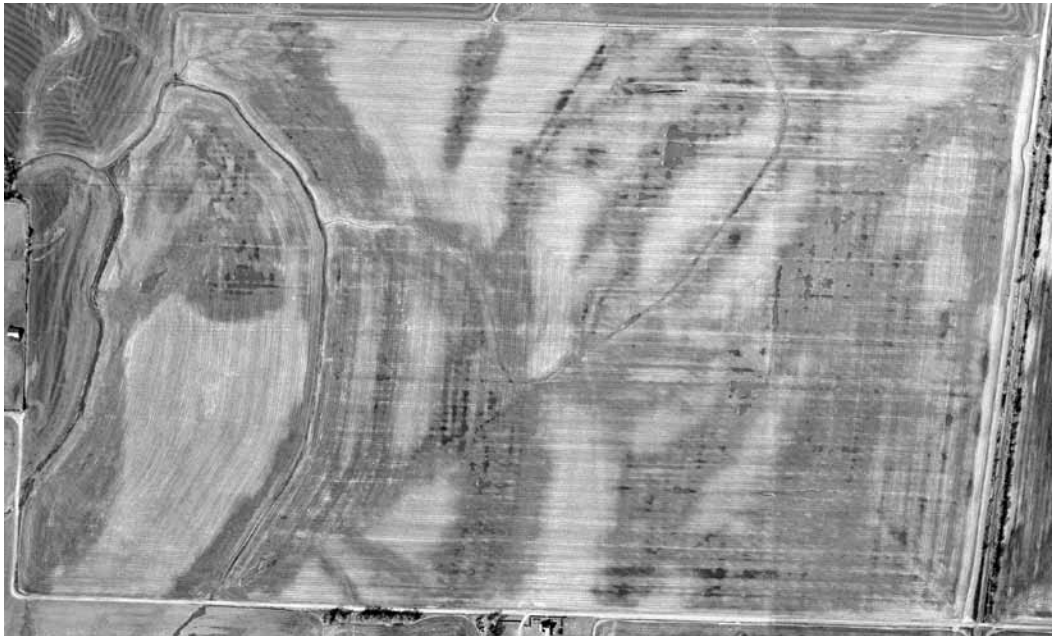
Figure 57. Aerial photograph of an agricultural field with saturated soils indicated by darker colors.
