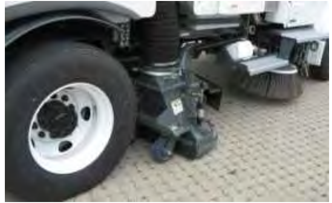
Routine, air-vacuum sweeping in the early spring and fall is the best approach for permeable pavement maintenance (Photo source: Toronto and Region Conservation)
