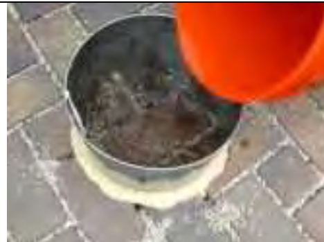
Infiltration test using ASTM C-1701
